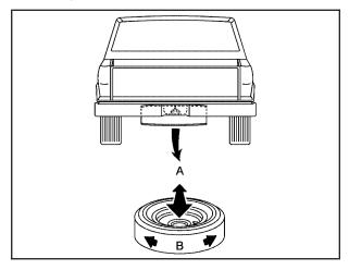
7. Make sure the tire is stored securely. Push, pull (A), and then try to turn (B) the tire. If the tire moves, check to make sure the tire valve stem is pointing down, then use the wheel wrench to loosen and then tighten the cable.
